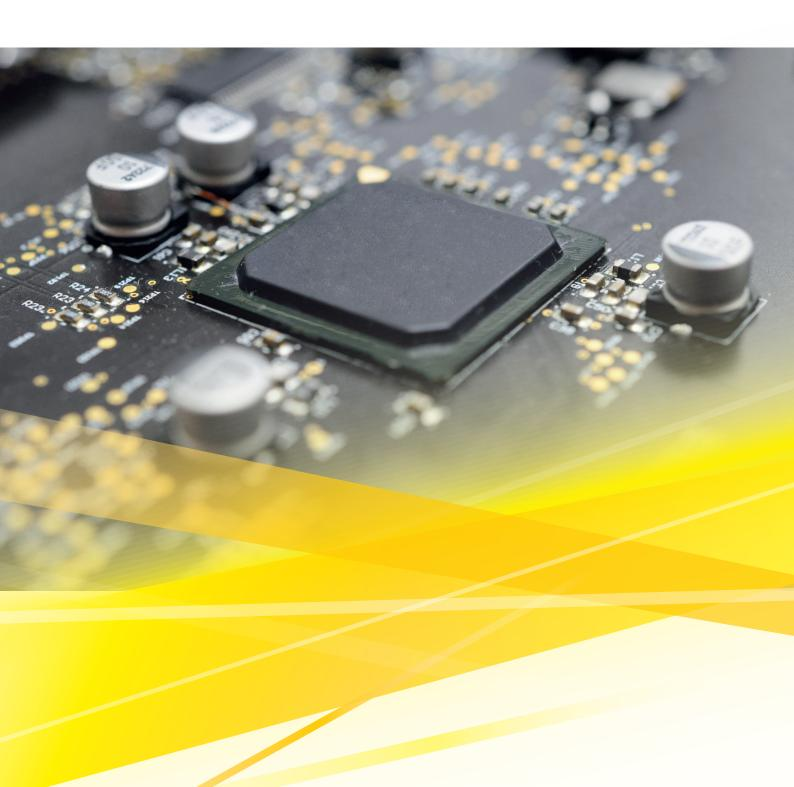
The Pantec Dynamics Drive Controller offers highest performance in drive control without the usual cost of flexibility. Based on FPGA (Field Programmable Gate Array) logic that allows control rates up to 200 kHz, multiple different motor types combined with various feedback systems as well as solenoid devices can be controlled.
